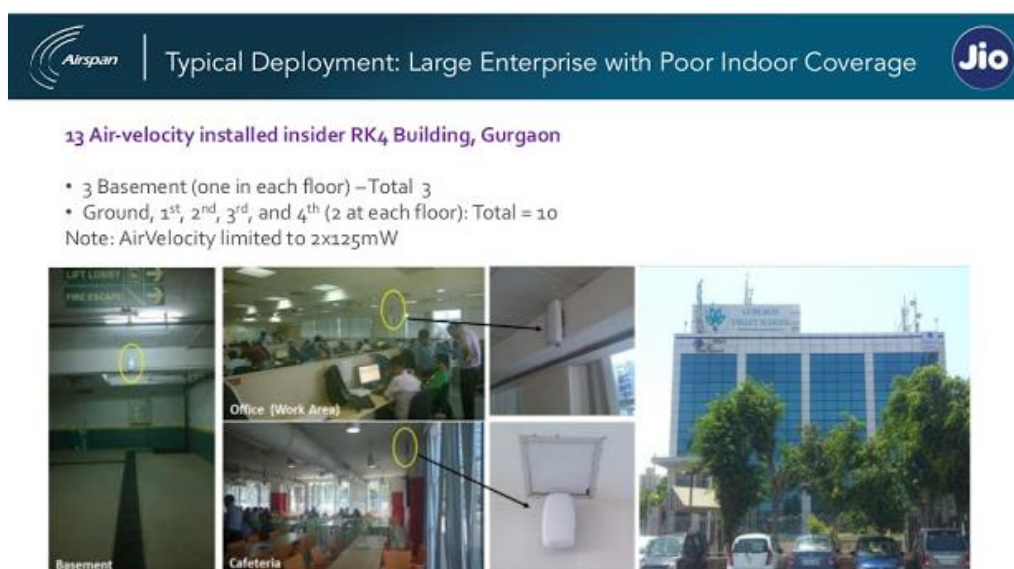
Figure 49 Example in-building deployment by Jio in Gurgaon, India (Source: Airspan)
